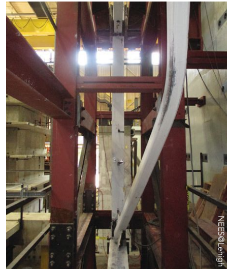
▲ OCBF brace buckling testing.
