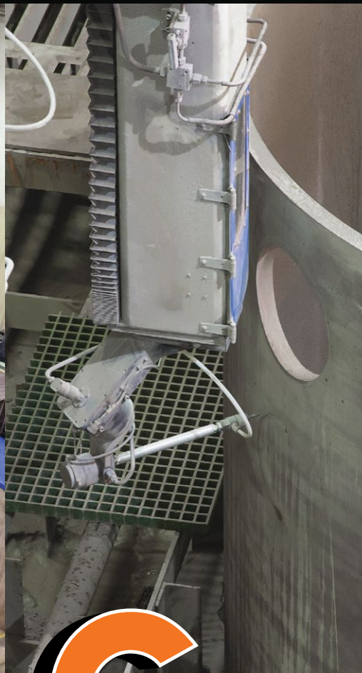
1.75-inch thick HY-80 Steel Plate rolled to 91.75-inch O.D. Holes cut into the cylinder after rolling. Thermal cutting not permitted.
