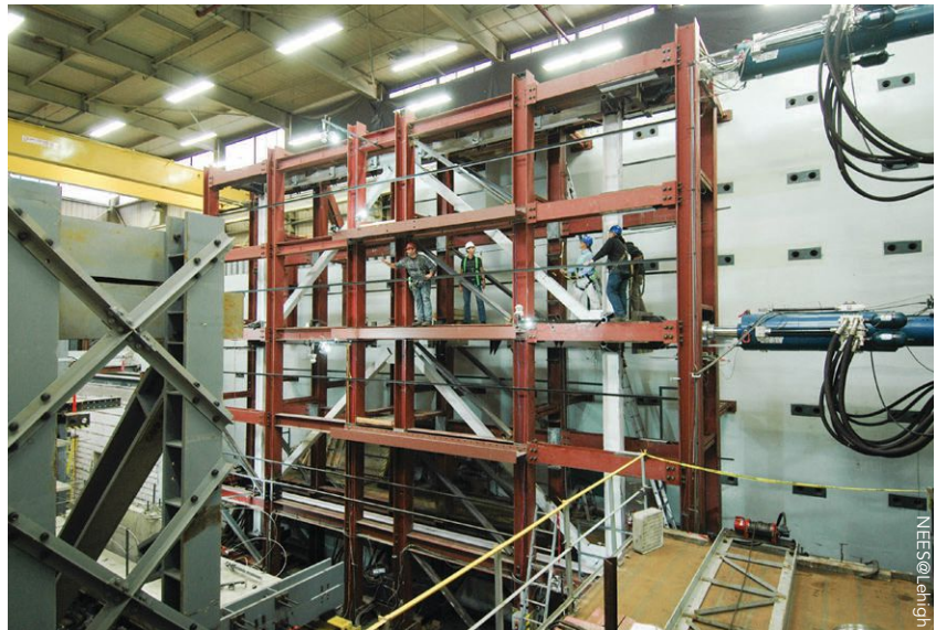
▼ R = 3 chevron braced frame testing.
