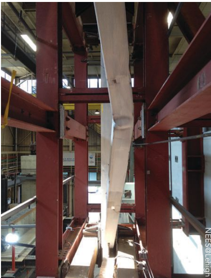
▼ R = 3 brace buckling testing.
